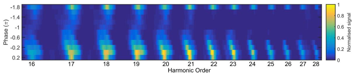
**Figure 1.** Experimentally observed high harmonic signal for different phases of the 2<sup>nd</sup> harmonic relative to the fundamental laser pulse. Tuning the phase controls the harmonic generation efficiency and the highest order observed which is directly linked to the dynamics of the relativistic electrons in the target.
