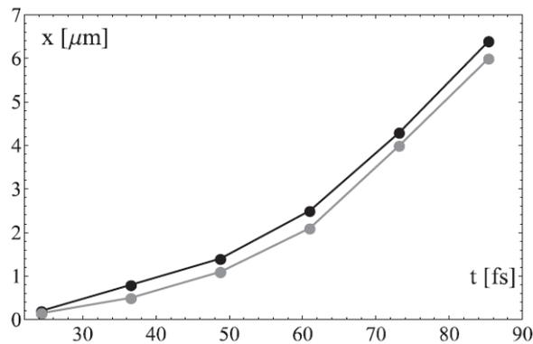
**Figure 1.** Synchronized motion of a laser pulse and a proton bunch: positions,  $x(t)$ , of the laser pulse front (gray) and the front of the accelerated proton bunch (black) inside a target
